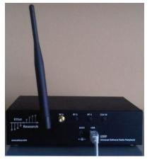
purpose Radio Frequency hardware device which provides a low-cost, readily but versatile radio functionality. It runs on the GNU radio platform.
