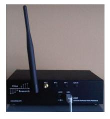
• USRP/USRP2: The USRP/USRP2 is a general purpose Radio Frequency hardware device which provides a low-cost, readily but versatile radio functionality. It runs on the GNU radio platform.
